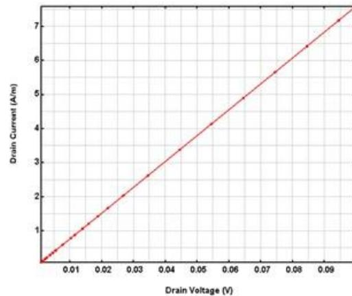
**Fig. 10  $R_{dson}$  characteristic.**
