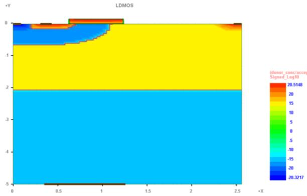
Fig. 5 LDMOS Simulation Structure.
