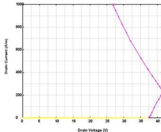
**Fig 14 LDMOS SOA Characteristic. The initial voltage scan is shown in gold. The continuing scan for the current boundary conditions is shown in violet.**
