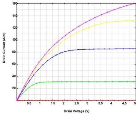
**Fig 8 Id-Vd Characteristic Curves.**
