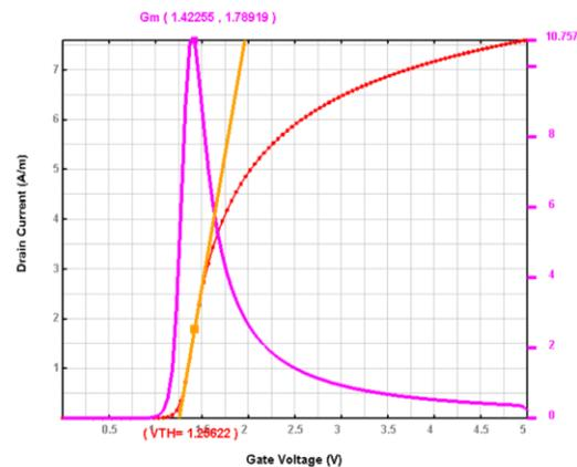
Fig 6  $I_d$ - $V_g$  Characteristic.
