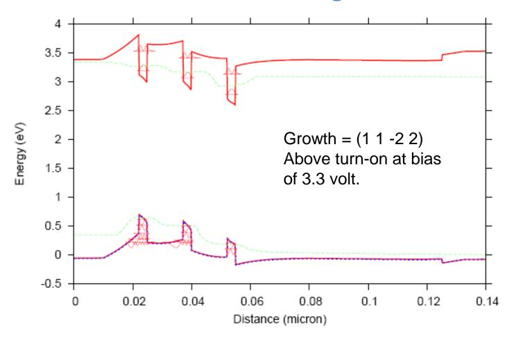
Simple 3MQW with optical gain spectrum imported from a separate active region calculation. Self-consistent simulation performed with internal field effects.
