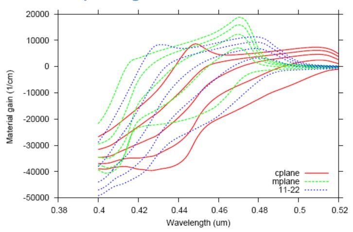
InGaN/GaN well with 20 percent indium; 3 nm well Well concentration from 3.e12 to 3.e13 (1/cm^2) in equal intervals Waveguide ridge parallel to projection of c-axis, TE polarization
