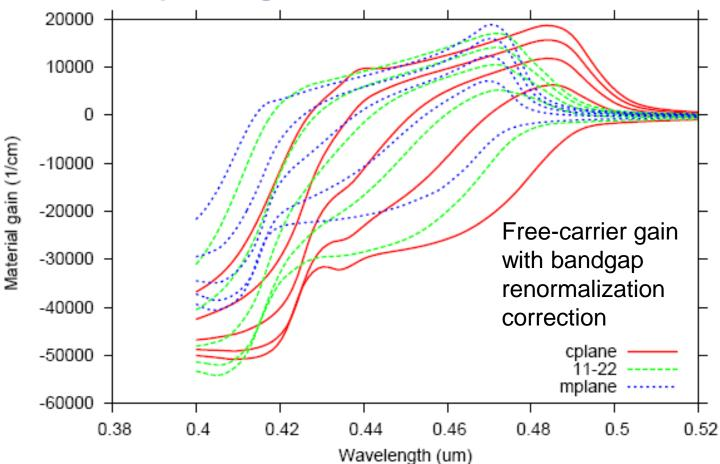
InGaN/GaN well with 20 percent indium; 3 nm well Well concentration from 3.e12 to 3.e13 (1/cm^2) in equal intervals Waveguide ridge parallel to projection of c-axis, TE polarization
