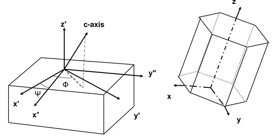
(x,y,z) – crystal coordinate where original Hamiltonian defined (x',y',z') – growth coordinate system; z'=MQW normal (x'',y'',z'') – waveguide system; z''/z'; y''=wave propagation direction
