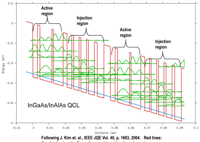
Conduction bands; Green lines: subband levels and envelop wave
