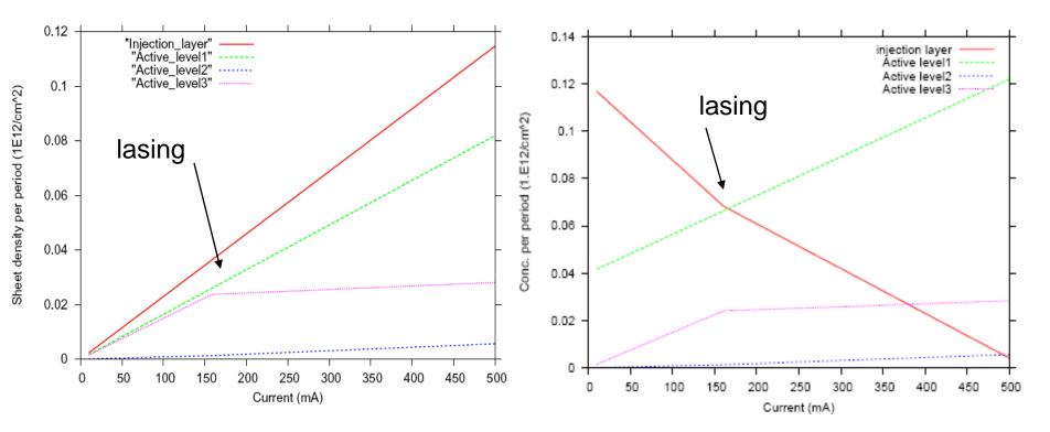
(a) Assume all tau's are constants and all levels are initially unoccupied. Current injection increases occupancy until lasing. (b) Assume injection region and active level1 are initially occupied.1/tau\_injection set to increase linearly with current to preserve total sheet charge.
